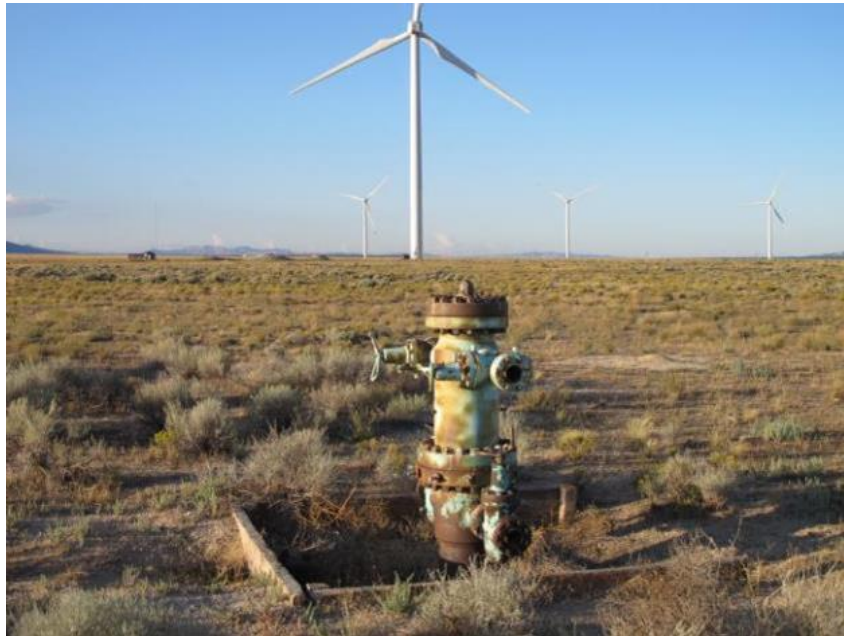
Figure 15a: Wellhead of Acord-1
